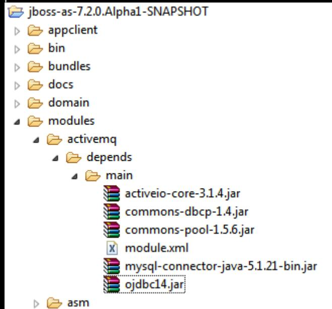
4. Create a file called module.xml in the same folder. This file needs to reflect the JAR files that Active MQ requires, to load successfully, and the JDBC drivers you intend to use.
